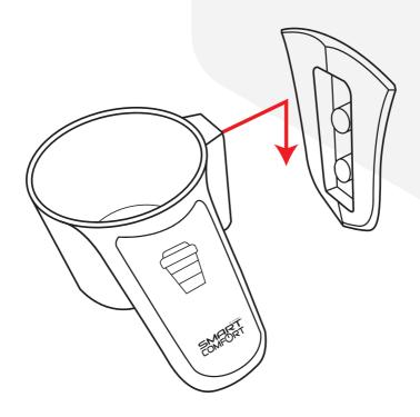
To install the cup holder, simply take the cup holder unit and line up the two holes with the two pegs on the chair's cup holder bracket. Allow the cupholder to slide downward to lock into place.
